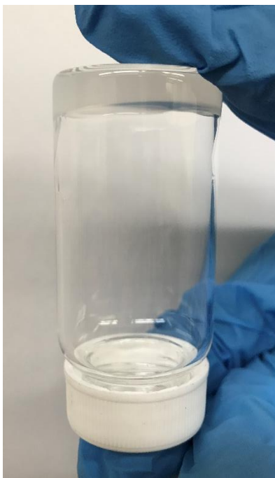
Figure S4. The translucent LiTFSI-HFE gel.
